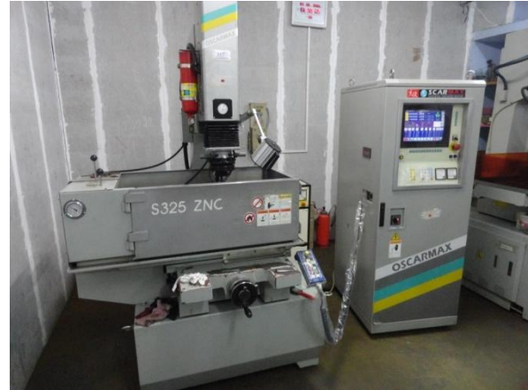
Figure.1. Experimental set up of EDM drilling machine
