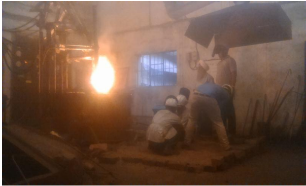
Figure 3.1 100 KVA SAF in Operation
