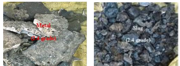
Figure 3.3 Alloy and slag sample collected after smelting
