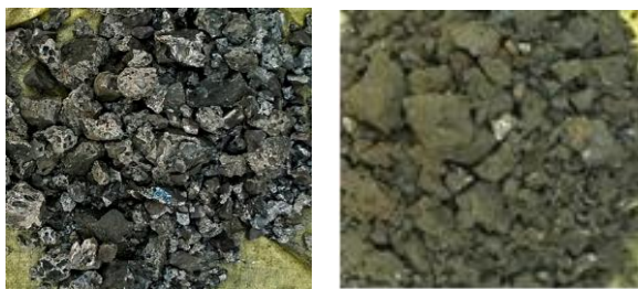
Figure 3.5 Alloy and slag sample collected after smelting of 2.8 grades Ferro-chrome
