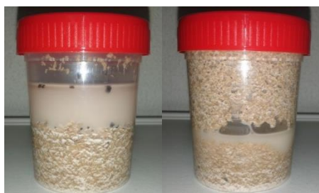
Figure 14 - Sedimentation of the two abrasive used in the formulation of the new product.
