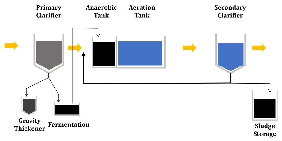
If Anaerobic Tank isn't really anaerobic ...
