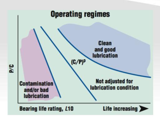
Relative effects of contamination and lubrication condition on bearing life with different load levels
