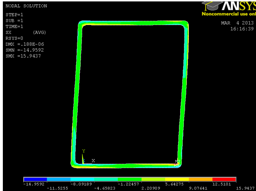
Figure 6: Stress concentration in cold-formed corners experiment
