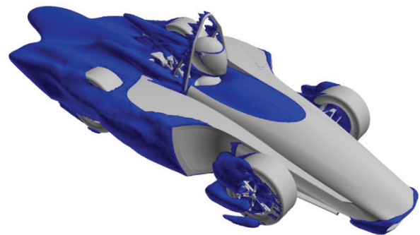
Figure 21. Iso surface of total pressure coefficient less than zero for case 3. Note that the recirculation zone in the sidepod that was discovered in case 1 and 2 is still present.
