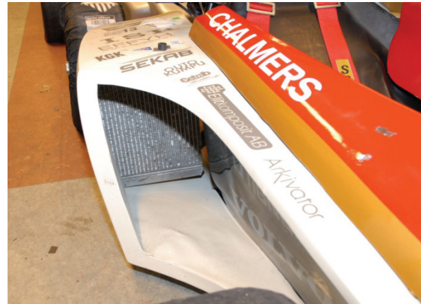
Figure 2. The original sidepod geometry of the Chalmers 2007 Formula Student entry.
