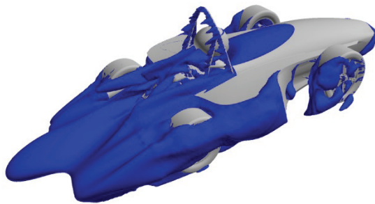
Figure 20. Iso surface of total pressure coefficient less than zero for case 3.
