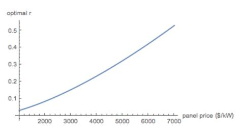
Figure 6. Effect of panel price on optimal variable rate
