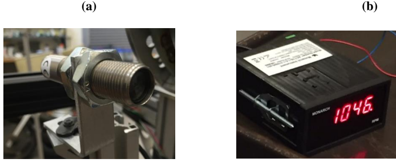
Figure 5.16: (a) Optical sensor for measuring the fan speed and (b) tachometer used to display the fan speed.
