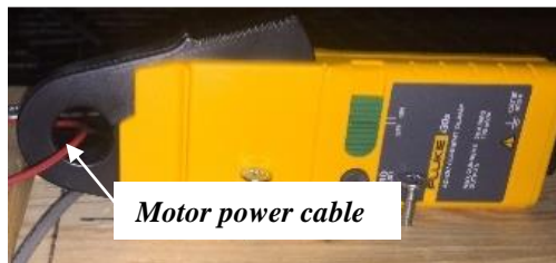
Figure 5.17: Current measurements of motor power cable using an i30s current sensor. Measurements are made by clamping the sensor around the cable.
