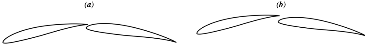
Figure 4.29: (a) E214-T2 airfoil geometry resulting in the best aerodynamic characteristics and (b) E214-T3 airfoil modified to accommodate for fabrication difficulties related to the proximity of the airfoils.
