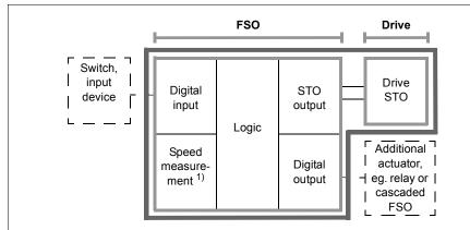
The safety data of the FSO and the drive is composed of the safety data of the subsystems used in the FSO and the safety data of the drive STO.
