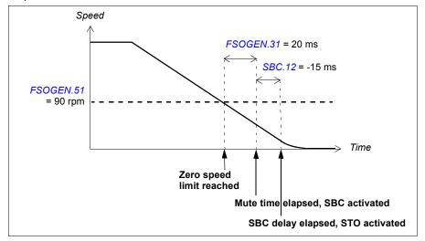
**Note**: If the SBC delay (parameter SBC.12 STO SBC delay) is positive or zero (0 ms), the SBC and STO functions are activated at the same time.
