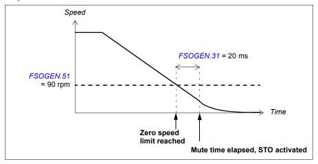
**Example 2**: Zero speed limit in reached in the SS1 function (and SSE with emergency ramp), a negative SBC delay (parameter SBC.12 STO SBC delay) is configured in the STO function:
