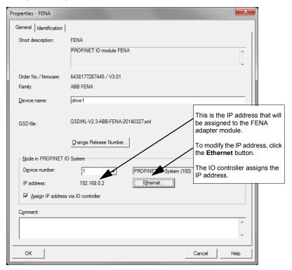
Note: Do not change the IP address assigned here. Use the same IP address for the FENA adapter module also in other tools (eg, the Drive composer pro PC tool) which you use to connect to the drive.
