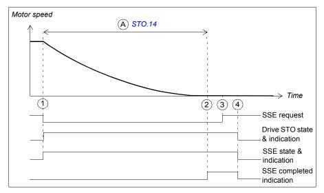
Time to zero speed (parameter STO.14): Time from the STO activation to the moment when the safety function is completed, the SSE completed indication (parameter SSE.22) goes on and the acknowledgment becomes allowed. You must set this to the estimated time in which the motor coasts to a stop from the maximum speed.
