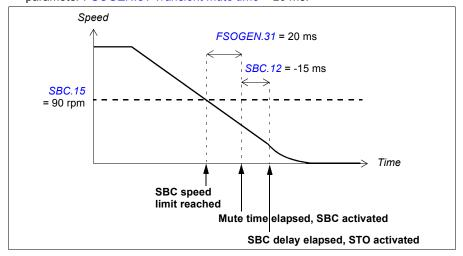
Note: If the SBC delay (parameter SBC.12 STO SBC delay) is positive or zero (0 ms), the SBC and STO functions are activated at the same time.
