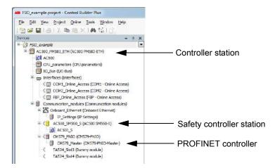
**Note**: Make sure that the "Enable debug" setting is On for the safety controller station, if you want to view or debug the PLC program after the download.
