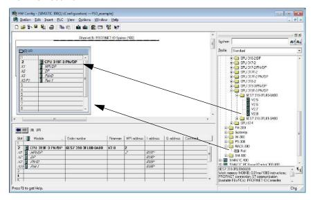
When you install the controller station to the rail, select Industrial Ethernet as the subnet for the controller station.
