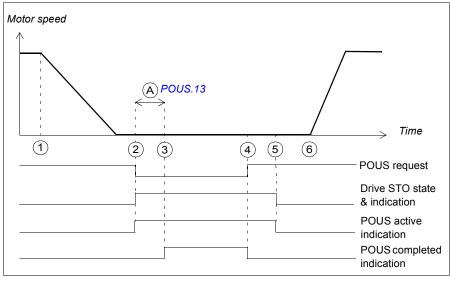
POUS delay for completion (parameter POUS.13): An additional security delay. The Α POUS completed indication (parameter *POUS.22*) goes on after this delay.
