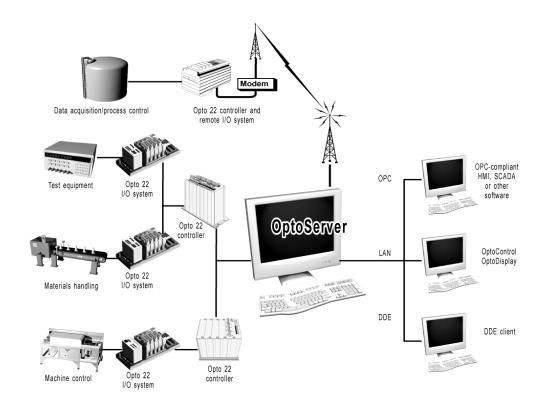
As you can see, several computer terminals, each running Opto 22, OPC-compliant, or DDE-aware clients, are networked to a PC running OptoServer. The PC running OptoServer has a direct physical connection to Opto 22 controllers via ARCNET, RS-485, Ethernet, or any other Opto 22 controller-supported communication option.
