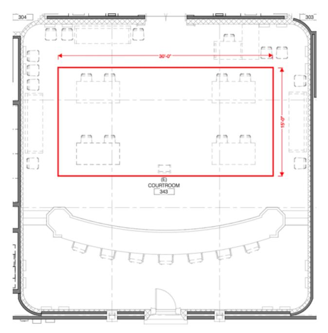
Plan view of courtroom with possible dimensions of floor covering. Diagram by Hennebery Eddy Architects.
