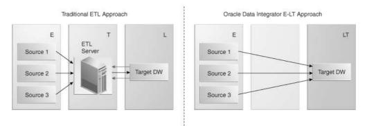
Figure 1: Traditional ETL approach compared to E-LT approach
