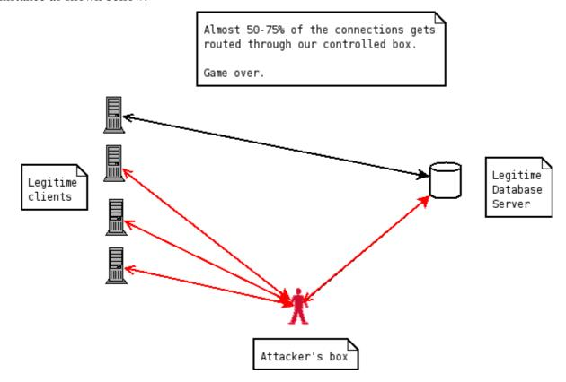
The clients connects to the attacker's controlled box which acts as a TNS proxy and forwards all connections to the legitimate database server, as shown in the picture. Not **all** the connections will be routed through the attacker's box as the TNS Listener will make load balance between all the established instances but, continuously registering the same instance will assure, at least, that the 50% of the connections will be routed through our controlled box.
