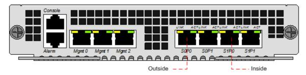
Plug the slot 0 port 0 (s0p0) interface into your Avaya facing gateway and the slot 0 port 1 (s0p1) interface into Cisco facing gateway. The slot 1 port 0 (s1p0) is connected to the Verint recorder. Once connected, you are ready to power on and perform the following steps.
