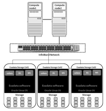
Figure 3.2 Eighth/Quarter Rack Exadata Database Machine compute and cell server architecture
