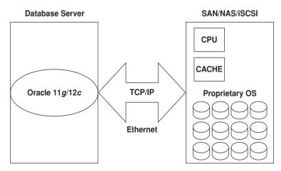
Figure 3.3 Traditional database and storage architecture
