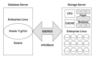
Figure 3.4 Exadata Database Machine architecture
