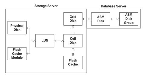
Figure 3.6 Exadata storage (physical, LUN, cell disk, grid disk, and ASM disks) formation flow
