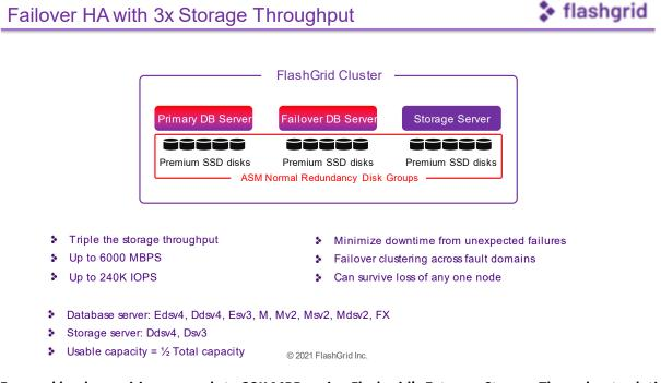
For workloads requiring upwards to 20K MPBs using Flashgrid's Extreme Storage Throughput solution:
