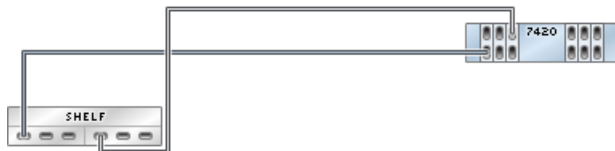
fig. 4 Standalone controller with six HBAs and one disk shelf in a single chain.
