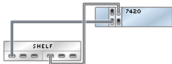
fig. 1 Standalone controller with two HBAs and one disk shelf in a single chain.
