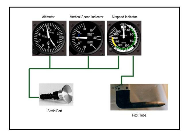
The Pitot-Static System drives the Altimeter, Vertical Speed Indicator (aka VSI), and the Airspeed Indicator. These instruments interpret air pressure.
