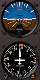
The Vacuum System powers the Attitude Indicator (aka Artificial Horizon) and the Heading Indicator (aka Directional Gyro or DG). These two gyroscopic instruments are of particular significance during flight in conditions of restricted visibility. If the Vacuum System fails, usually due to a failed vacuum pump, these two instruments will gradually begin to fail as their gyroscopes slow to a stop.
