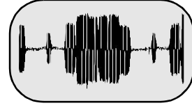
③ 5.36V p-p IC3001 PIN 34 C_IN
