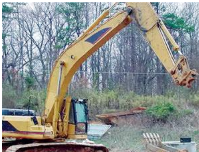
Figure 1. Quick-disconnect excavator bucket that detached from the excavator stick.
