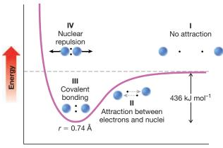
**FIGURE 1.9** The potential energy of the hydrogen molecule as a function of internuclear distance.
