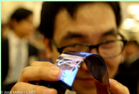
Figure 3. Building better OLED displays. Left: Samsung has announced the near-future release of a foldable smartphone built with a flexible plastic OLED display; the phone can be folded to an eighth of its size. Source: Josh Miller/CNET. Right: Both Samsung and LG Electronics have announced near-future releases of 55-inch, 4-mm thick OLED display TVs. Source: LG Electronics.
