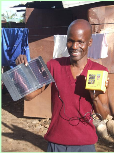
Figure 7. Accessible electronics. Pay-as-you-go organic solar cell technology is being distributed throughout rural areas of southern Africa and elsewhere, providing a low-cost and safe alternative to kerosene. Source: Eight19.
