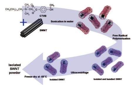
Figure 1. Schematic view of the procedure to fabricate *p*-SWNT.
