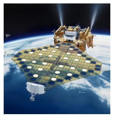
Miura-ori Solar Array designed by Koryo Miura (Japanese), Japan, 1995, illustration by T. Mizuno, courtesy of JAXA
