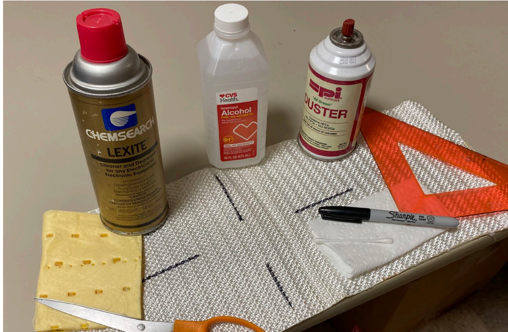
Figure 2 – Photograph of cleaning supplies and drafting equipment for aligning target as a reference on the geosynthetic
