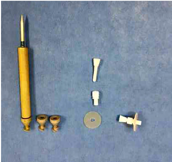
Figure 2. Portals with a suitable design for varying the diameters of the ultrasonic probe. Source: The Author (2018)
