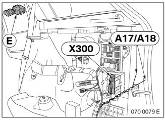
Connect connecting point to plug **X300** of PDC electronic control unit with miniature connector **E** as follows:
