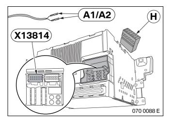
Make the pinning in plug **X13814**, 12-pole, WS, as follows:
