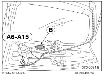
Thread connecting points **A6** to **A15** to the installation point of rear-view camera **B** as shown in the picture.
