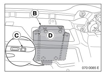
Insert camera **B** with lens into rubber seal **C** from the inside. Secure camera **B** with two Torx bolts **D**.
