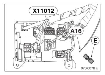
Pin connecting point **A16**, RTGN, into plug **X11012**, GR, PIN 8 from fuse carrier luggage compartment.
