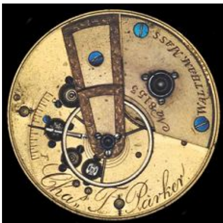
Figure 18. 15J Chas T. Parker 8153 with real jewel settings and 11J P.S. Bartlett 8406 with burnished jewels (Photo of P.S. Bartlett 8406 permission of Hans Dahlke)
