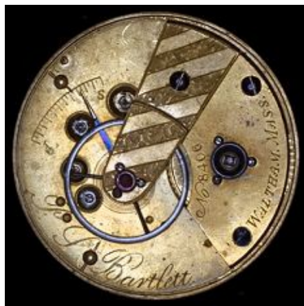
Figure 18. 15J Chas T. Parker 8153 with real jewel settings and 11J P.S. Bartlett 8406 with burnished jewels (Photo of P.S. Bartlett 8406 permission of Hans Dahlke)
