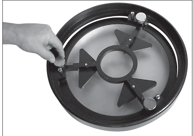
Figure 36. The tilt of the primary mirror is adjusted by turning one or more of the three collimation knobs.
