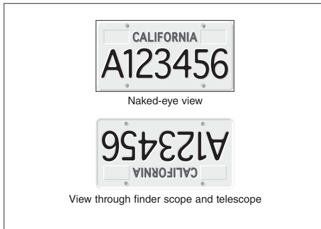
Figure 40. The view through a straight finder scope and reflector telescope is rotated 180°. This is true for the XX12 and its finder scope as well.
