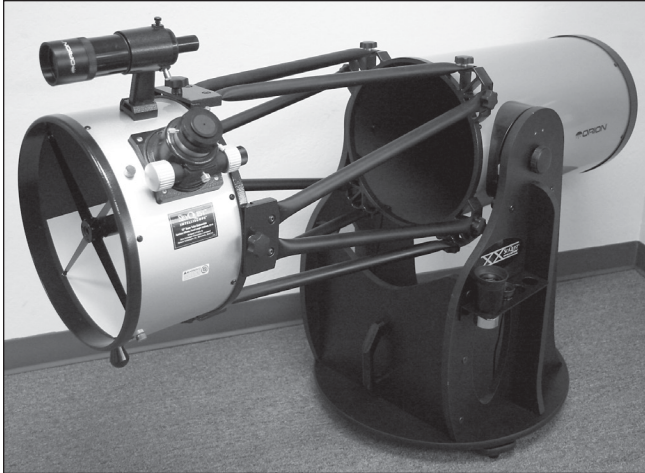
Figure 32. This image shows the XX12 properly set up for collimation. Note the white paper placed across from the focuser and the level angle of the optical tube. Ideally, the telescope should be pointing at a white wall.
