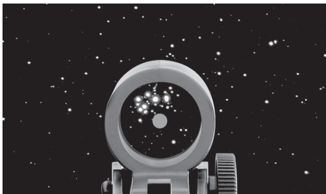
Figure 5. The EZ Finder II superimposes a tiny red dot on the sky, showing right where the telescope is pointed.
