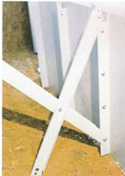
This brace, installed every 4', coupled with the vertical Z-bar® stiffeners – welded every 2' – gives your X-Brace™ pool outstanding strength. This Fox-created design concept has been imitated but not duplicated. All Fox claims are backed – in writing – in a detailed Engineering report.
