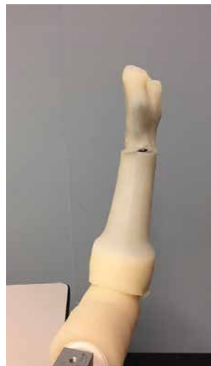
Figure 1. Wrist fracture simulator
