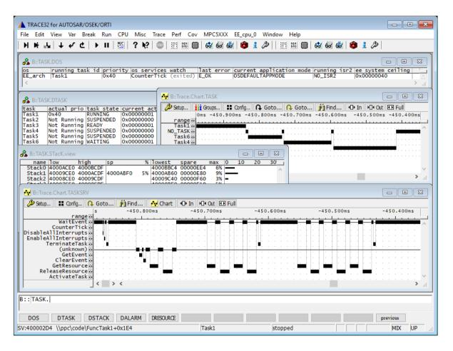
The OSEK Run Time Interface (ORTI) is a specification, which enables debuggers to become OS-aware, without knowing the OS itself. Most AUTOSAR/OSEK system builders are able to extract all necessary information of the OS component into a text file, called "ORTI file".
