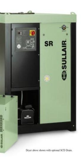
These dryers cool compressed air by mechanical refrigeration, removing the moisture and assuring that none condenses downstream, unless the air is exposed to lower temperatures. With models ranging from 5 to 3000 scfm (.15 to 85 m³/min), you can specify an SR dryer that is virtually customized to your requirements.
