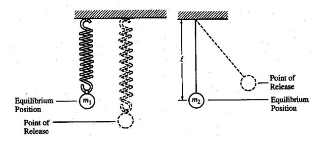
A sphere of mass m<sub>1</sub>, which is attached to a spring, is displaced downward from its equilibrium position as shown
