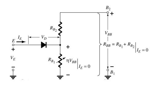
The equivalent circuit indicates that the UJT is like a diode and a resistive voltage divider circuit. The resistance exhibited by  $R_{B1}$  is variable; it is dependent on the value of current  $I_E$ .
