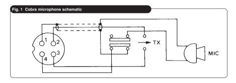
If the microphone to be used is provided with pre-cut leads. they must be revised as follows.
