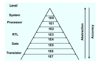
Figure 1.2: Levels of abstraction in SoC design (source [18])
