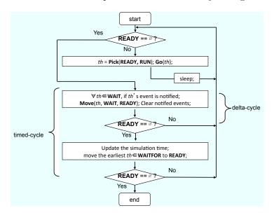
Figure 3.1: Traditional sequential Discrete Event simulation scheduler
