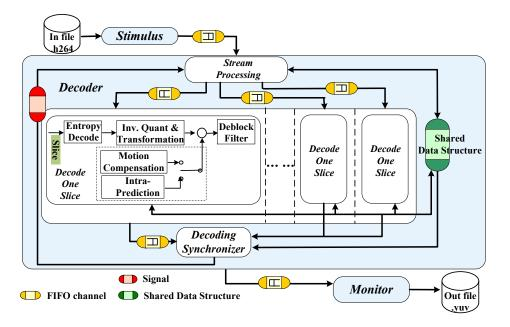
Figure 2.3: Proposed H.264 Decoder Block Diagram
