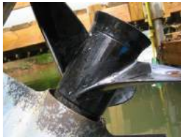
Fig. 4 Vortex “C” Series (3-3/8”) Propeller installed on a V4 (4-1/4”) gearcase. Results in poor performance and excessive ventilation. Vortex “B” Series (4-1/4”) Propeller should be used.
