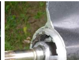
The shaft taper takes forward thrust from the thrust washer. Without a forward thrust washer, the gearcase takes the forward thrust as the propeller will continue to move forward on the shaft, causing severe damage to the gearcase.
