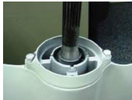
Fig. 5 Propeller shaft taper is visible, indicating OEM forward thrust washer has been removed. XHS Hub Kit forward thrust washer ready to be installed.
