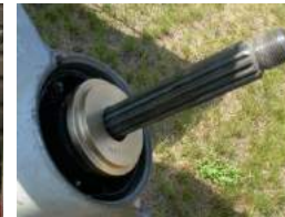
Fig. 7 The forward thrust washer is tapered and will nest with the taper on the propeller shaft. When properly installed, the part number will be visible.
