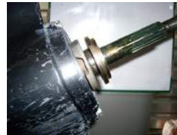
Fig. 6 OEM forward thrust washer was not removed. XHS Hub Kit and Michigan Wheel propeller will not fit properly.
