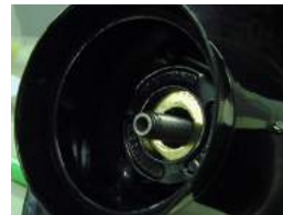
Aft drive adapter incorrectly installed. The propeller will fall off the propeller shaft if run with this incorrect installation.
