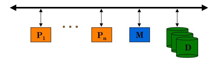
Examples : symmetric multiprocessors (Sequent, Encore) and some mainframes (IBM3090, Bull's DPS8)
