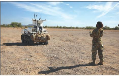
U.S. Army Spc. Destiny Jones, navigates a Robotic Combat Vehicle during Project Convergence at Yuma Proving Ground. The Next Generation Combat Vehicle Cross-Function Team is experimenting with using the vehicle for semi-autonomous resupply, helping Soldiers get the materials they need on the battlefield. (Photo by Spc. Kayla Antsey)
