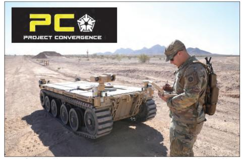
U.S. Army Pfc. Daniel Candales, assigned to the 82nd Airborne Division, uses the tactical robotic controller to control the expeditionary modular autonomous vehicle as a practice exercise in preparation for Project Convergence at Yuma Proving Ground. During Project Convergence 21, Soldiers are experimenting with using the vehicle for semi-autonomous reconnaissance and re-supply. (Photo by Sqt. Marita Schwab)
