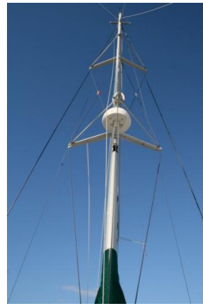
Outremer 45 radar on mast
