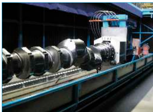
MT UNIMAG 13000 for shafts testing up to 25t
