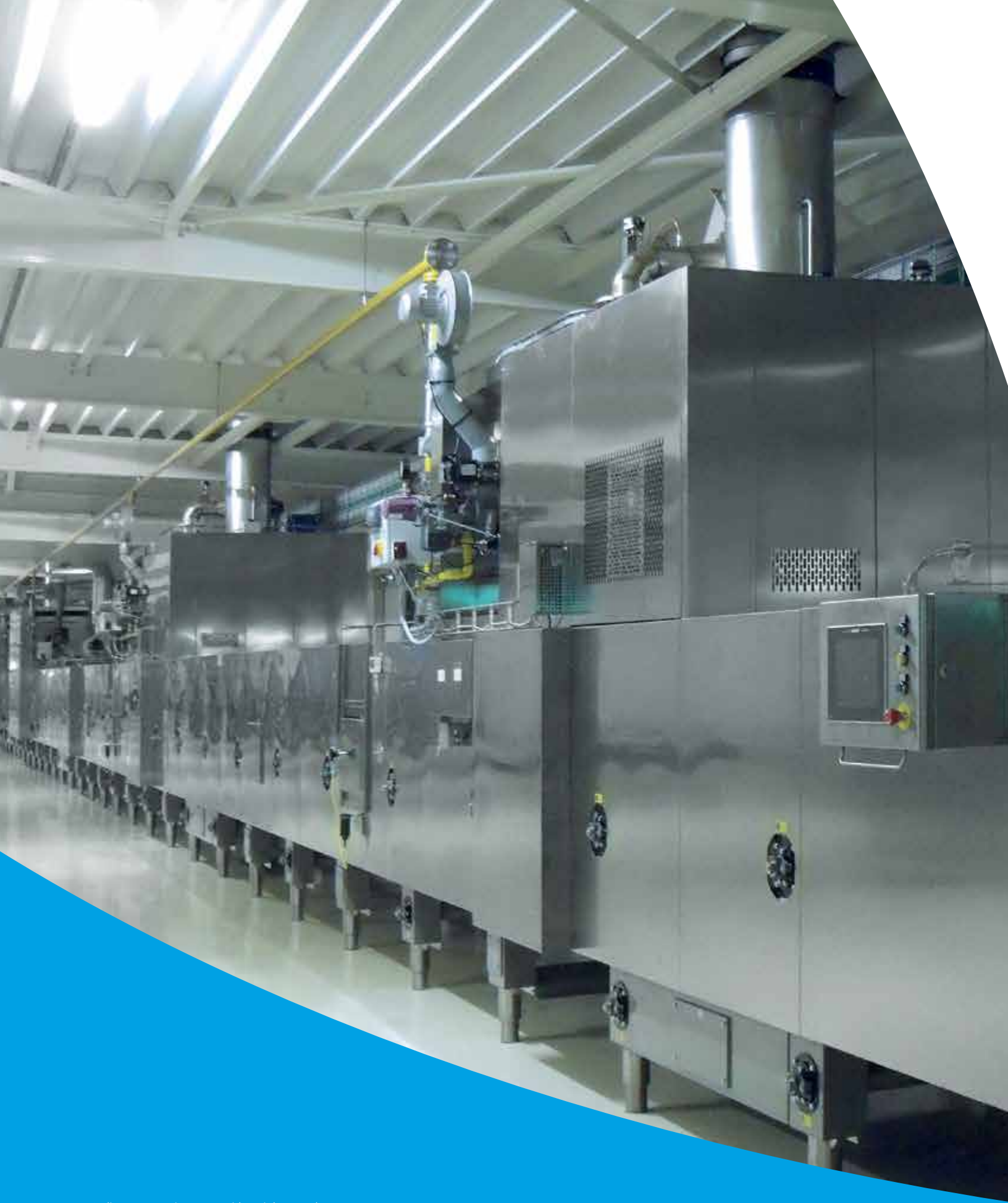
Indirect convection oven with stainless steel covers
