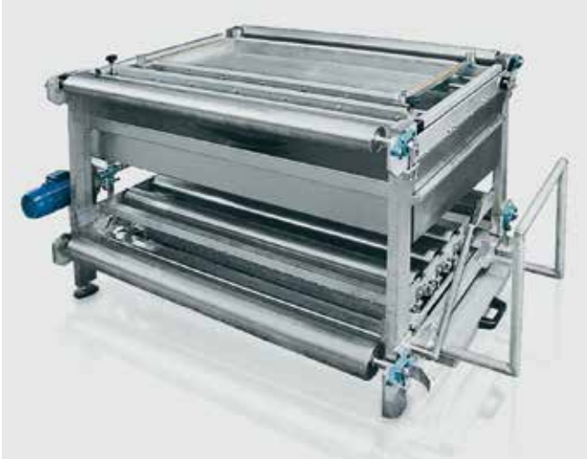
When space is tight, a band water cooling system can be installed at the oven outfeed. This setup helps to ensure that products are not damaged when they are detached from the oven band
