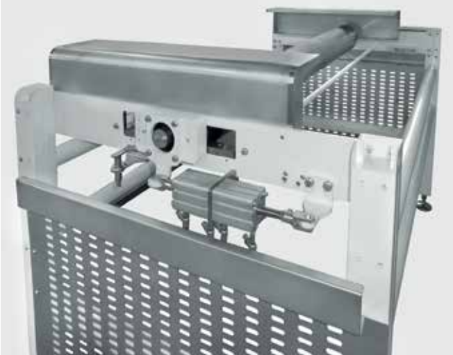
An automated pneumatic tracking system for the oven conveyor provides accurate conveyor speed and transit through the oven
