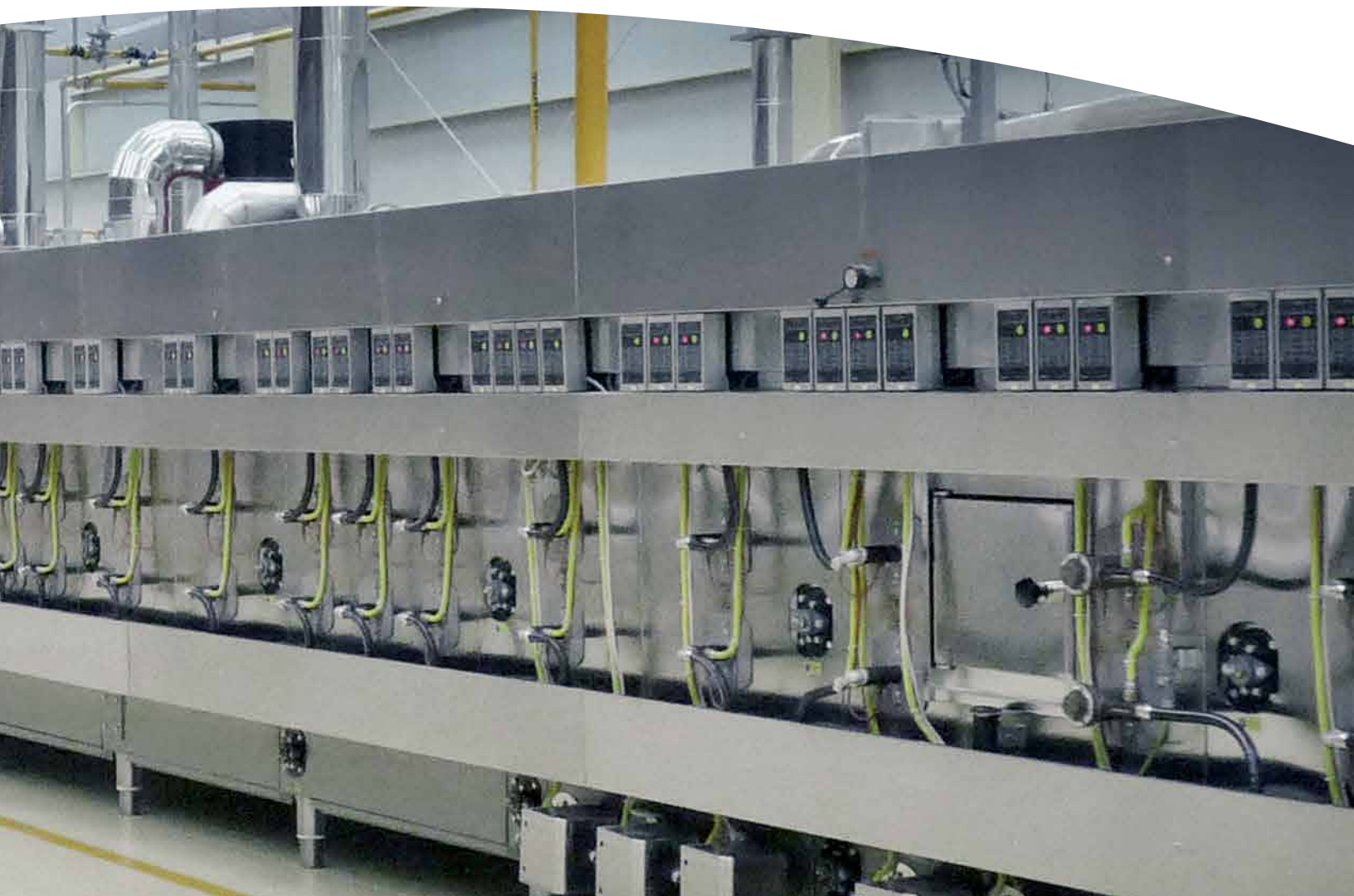
The flame height can be adjusted differentially across the width of a tri-zone burner to precisely control heating
