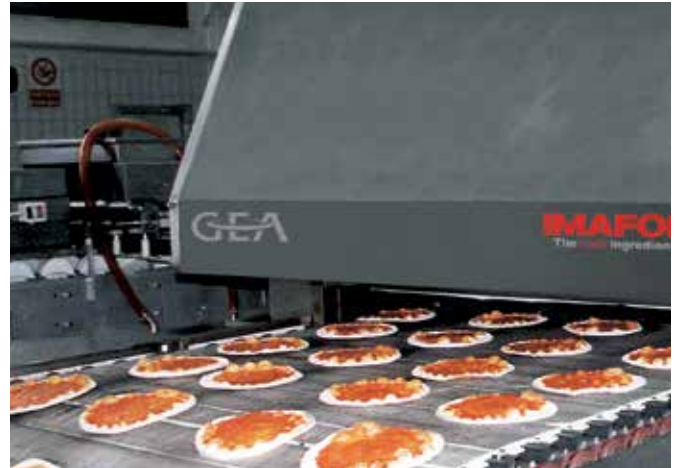
A special oven with a stone-based conveyor, which will bake perfect pizzas at the required high temperature and fast transit time
