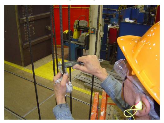
Properly inspecting the rope, and keeping an eye out for changes in the rope, is important to maintaining a safe work environment.
