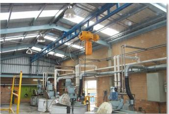
A type of overhead crane that travels suspended on a single rail.
