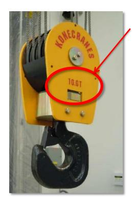
Load Markings are posted on all sides of the crane and on the hoist block.
