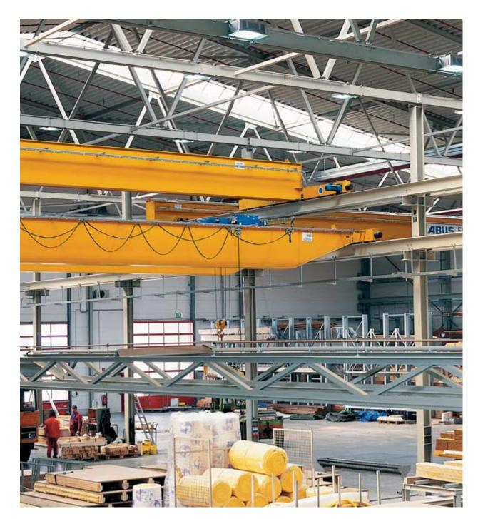
If a certain lifting height is only required in part of a hall, ABUS travelling cranes can be installed on different levels. In this example, an ABUS ELS single girder torsion box crane is used on the higher level, with an ABUS ZLK double girder travelling crane with a DQA ultra low headroom hoist on the lower level. This configuration ensures the safety distance required and maximises the available lifting height.
