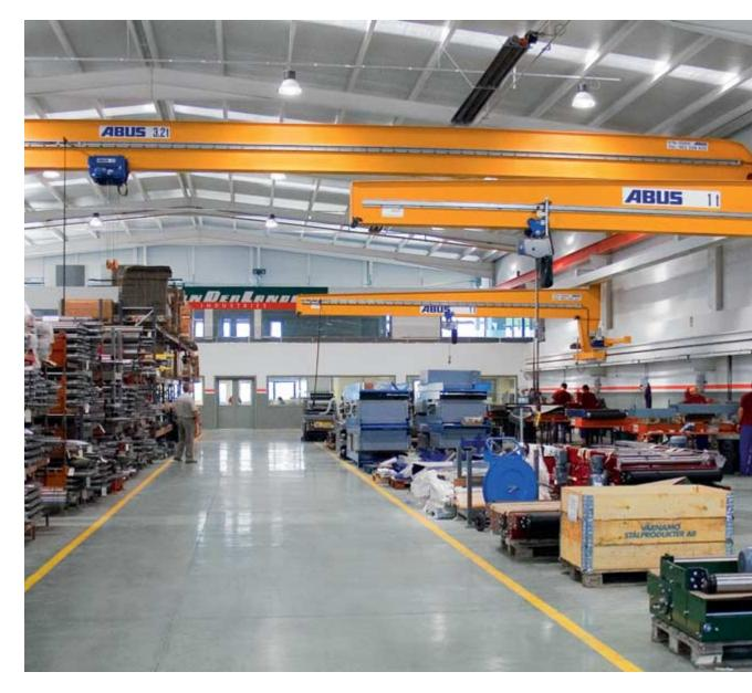
The ABUS single girder wall travelling crane is designed for operation on a lower level beneath a large travelling crane system. These cranes provide additional handling possibilities and ensure smooth and troublefree material handling between different working areas. A wall travelling crane installed at right angles across the hall can serve several working stations. ABUS single girder console travelling cranes are available for load capacities up to 5 t with track lengths up to 12 m.
