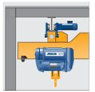
Standard main girder connection configuration Version 1, "angled" (variable overhang for minimum side approach dimension)
