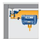
Stooled up configuration Version 2 (optimised hook height without crane girder cantilevers)
