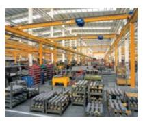
ABUS single girder travelling cranes ensure efficient material handling even where very little space is available in production halls or warehouses. ABUS single girder travelling cranes are available with rolled section or box girders. Each model is available in different girder connection versions to allow a space-saving configuration and an optimised highest hook position.
