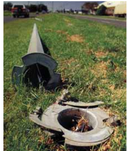
Figure 8.3: Frangible lamp post after vehicle collision, Australia
