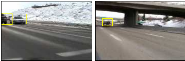
(c) Partial occlusion of two overtaking vehicles. (d) Illumination changes due to passing through the overpass.
