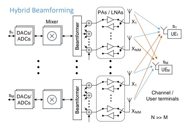
Digital beamforming/mMIMO is used at sub 6GHz frequency bands today Hybrid beamforming is used at mm-Wave frequency bands today
